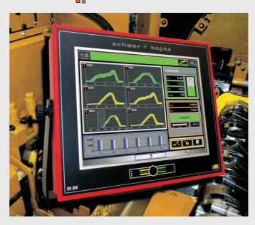
The SKHot*master* Module for monitoring hot forging machines is available in our process monitoring systems with built-in computers.
