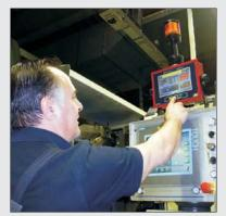
All thread rolling machines and a number of secondary machines are equipped with the compact monitoring terminal **SK 400** featuring a 7" touch screen.
