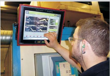
A single terminal serves both, data collection and load monitoring functions on all cold forming machines at ABC **SK-Reporter** up-to-date information provided by Schwer + Kopka GmbH
