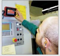
Entering a down code at the **SK 200 T** data terminal on an assembling machine
