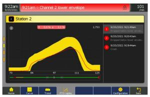
The PTO Replay feature brings single functions of the Process tracking office (PTO) directly to the device. This function allows the operator to analyze process error curves and their progression through a small movie.
