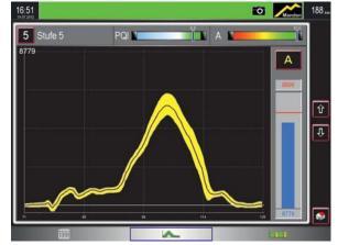
The Mandonic auto enveloping system adjusts the envelope limits perfectly according to the current variation of the process. The result: reliable detection of process errors with virtually no unnecessary machine stops. SKPuzzlemaster is provided for quick activation of additional expert monitoring routines.
